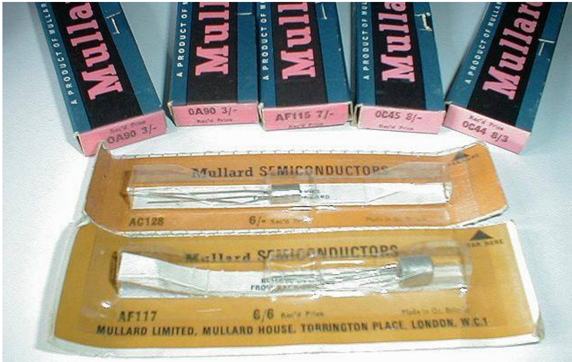
Above: New old stock (NOS) 1960's-vintage germanium semiconductors resplendent in their original packing. Note the prices, ranging from 3 shillings (15p or 30c) for the OA90 point-contact diodes, to a whopping 8 shillings and 3 pence (42p or 84c) for that 'exotic' OC44
