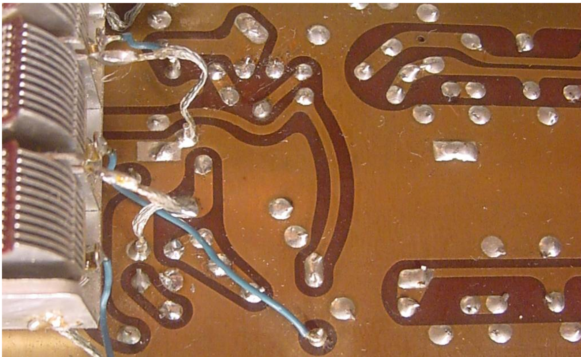
Above: the off-dreaded printed circuit board construction – shown here is the print side of the RF board in my EC10 MkI following replacement of the Mixer and Local Oscillator transistors
