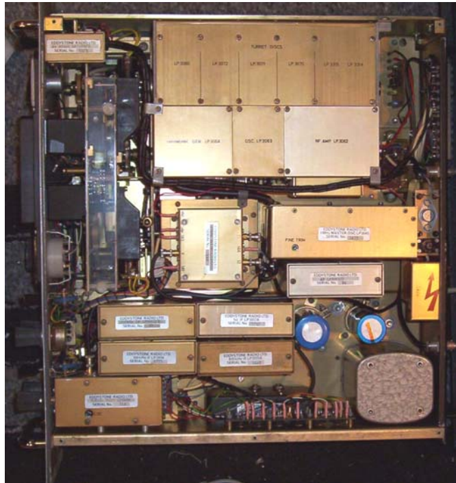
My EC958/3 with the case removed– modular beauty at its finest... here viewed from the top
