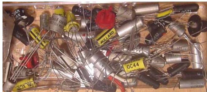
Junk box germanium small-signal transistors – some NOS, but mostly recovered from scrapped 'trannies'
